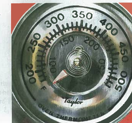
FIGURE 17-6 Photograph of a thermometer using a coiled bimetallic strip.
