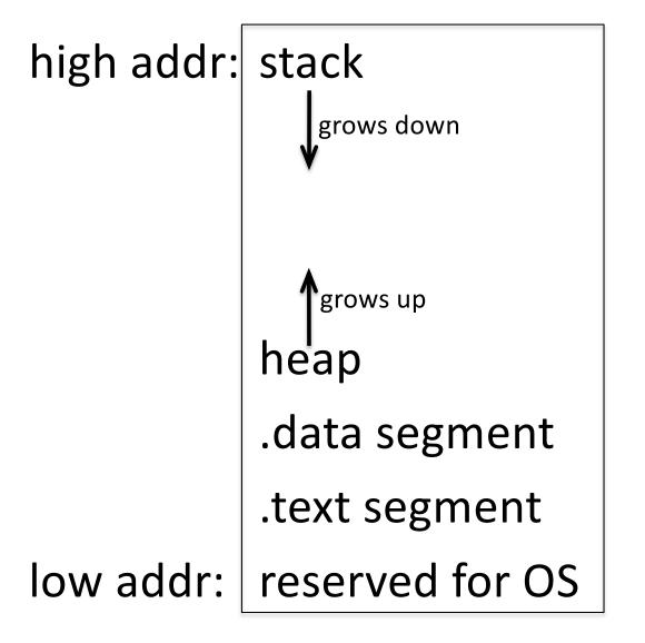
Stack composed of "activation records" or "stack frames", each with the local variables and saved registers for one function call
